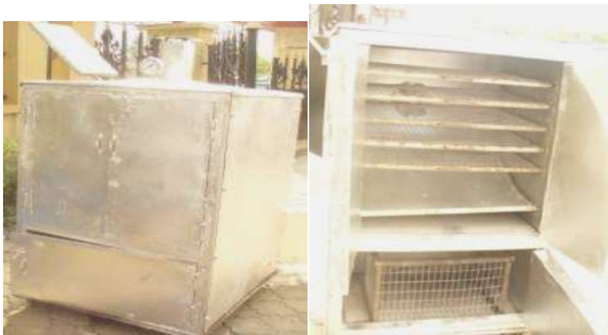
Plate 1: Improved NIOMR Fish Smoking Kiln
